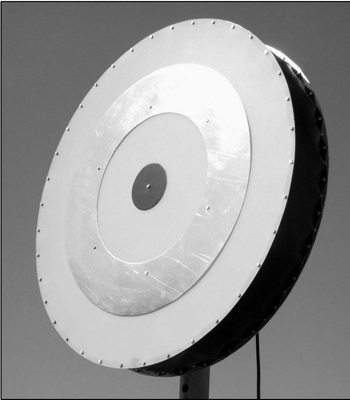
Fig 42: Archery target antenna prototype.
